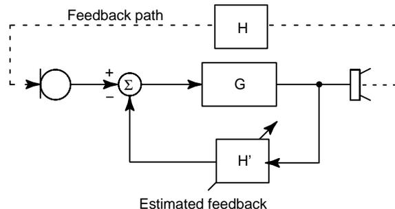
**Figure 5. Adaptive Feedback Canceller (AFC) Block Diagram**
